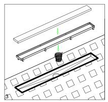
STEP1. Assemble the supporters under the tray (as shown in picture1), ensure it is seated properly. Then turn the opening frame of the tray upwards for use.
