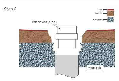
2.If there is a gap, mark the appropriate length on the extension pipe, cut it properly, and use glue to connect it to the waste pipe.
