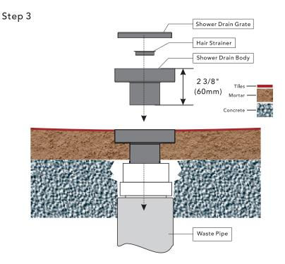
3. Finally, evenly apply waterproof fixing material around the area, place the floor drain, press it firmly, and clean off the excess material to complete the installation.
