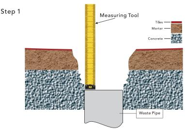
1.Use a measuring tool to check if the depth of the waste pipe meets the required installation depth for the shower drain body. The top of the waste pipe must extend into the bottom of the shower drain body by 1"(25mm) - 1 1/8(28mm)".
